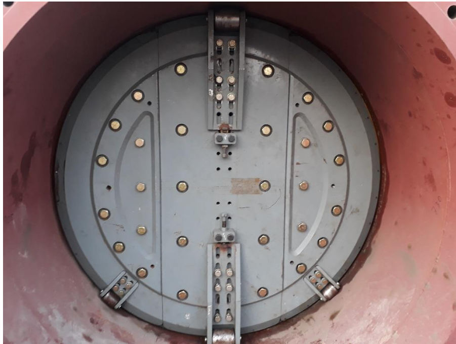
66" Folding plugging head on test prior to deployment
