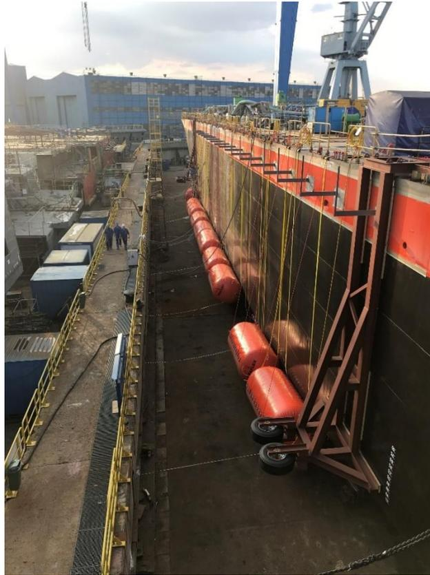
Some of the 42 x 20t Seaflex IBUs installed on the hull within the drydock prior to tow-out
