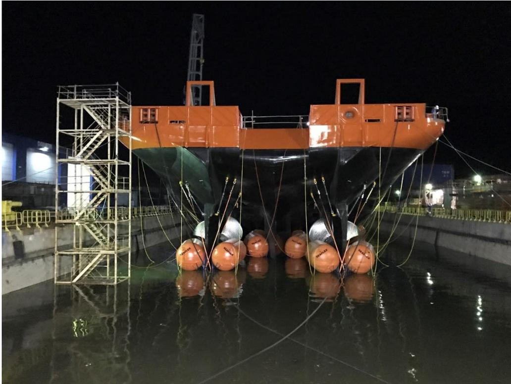
As the water level rises, the 20t Seaflex IBUs begin to support the weight of the hull
