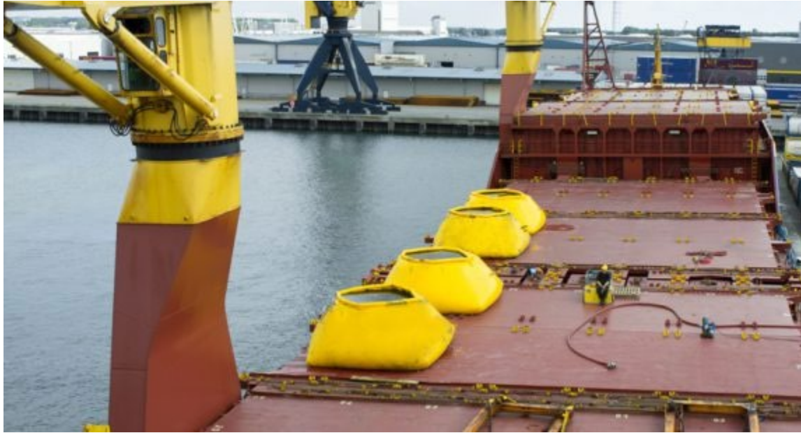
Our 25-tonne flexidams placed on the cargo vessel for an inclining test
