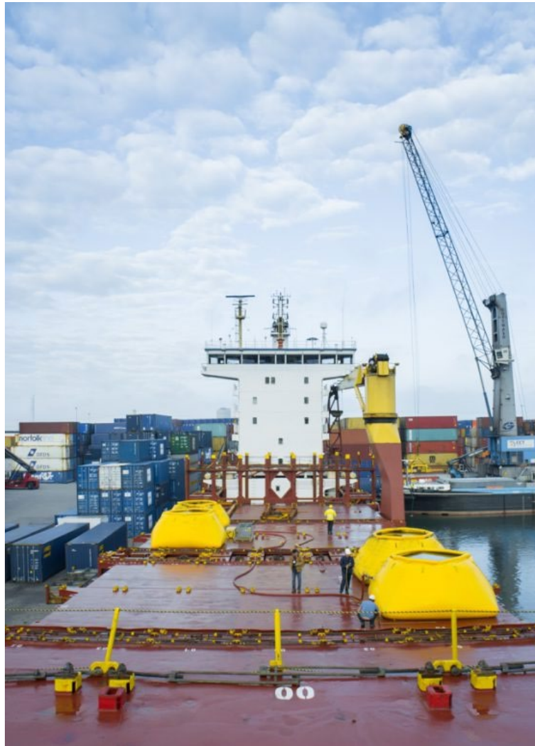
The flexidams were moved along the vessel during the duration of the test
