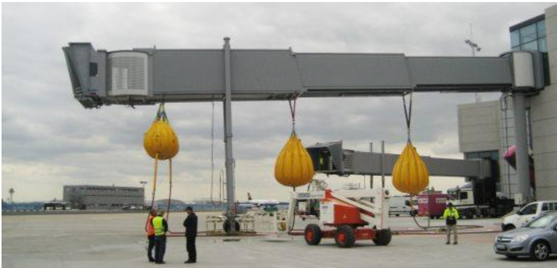
Water-filled proof load bags used to test the passenger bridge
