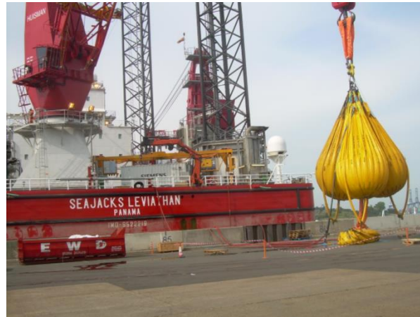
Water-filled proof load bags in use during the test
