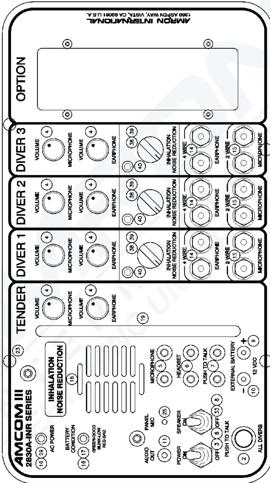
6.2 PARTS IDENTIFIER, MODEL 2830A-09, WEATHER RESISTANT AC POWER
