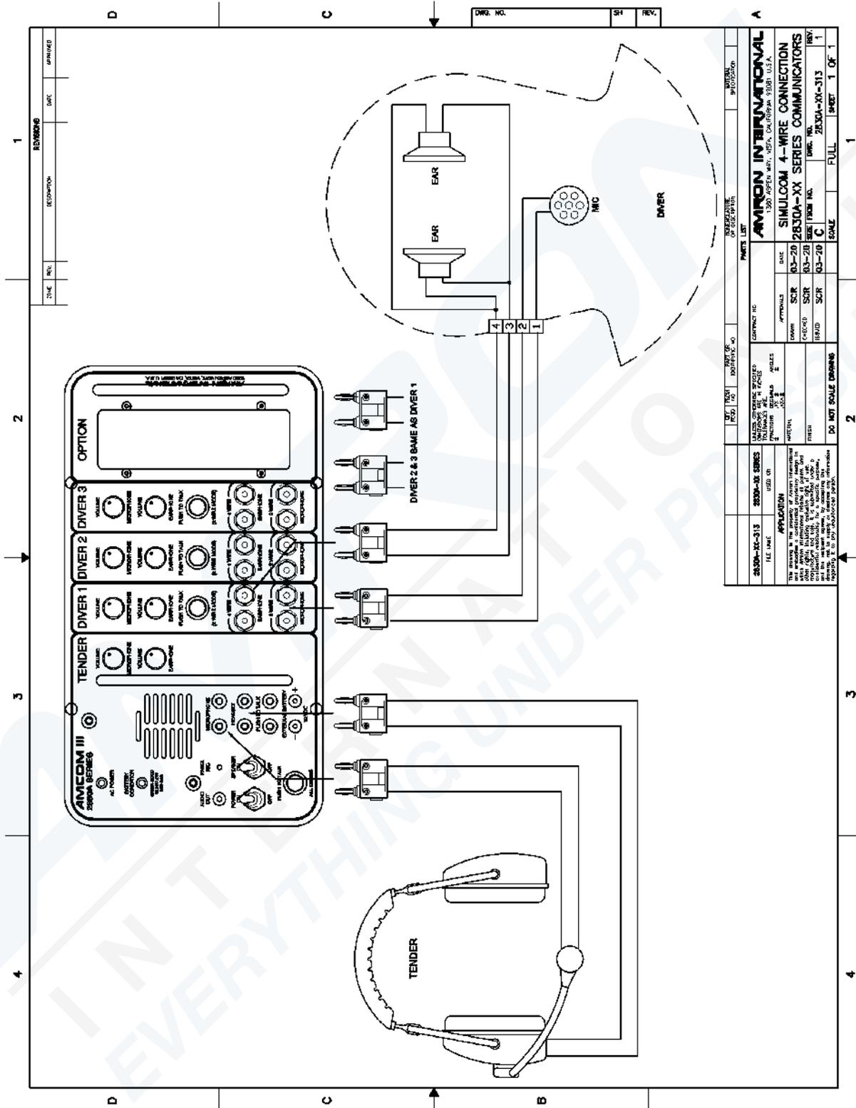
3.8 DRAWING, OPERATOR CONNECTIONS, HAND HELD MICROPHONE
