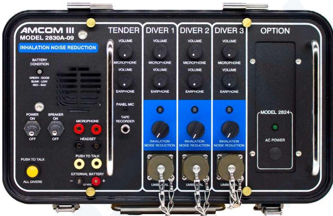
Amron's INR module features an individual inhalation noise reduction circuit for each diver that can eliminate inhalation noise completely or suppress the inhalation noise to the degree the operator demands. The net result is improved communications and intelligibility between the tender and divers.
