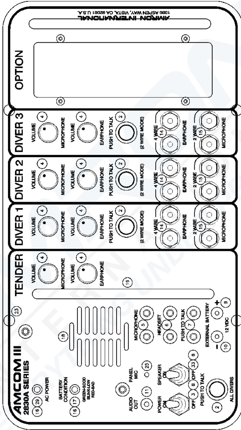
6.5 PARTS IDENTIFIER, MODEL 2830A-12, WEATHER RESISTANT AC POWER MODULE & DSP3 HELIUM SPEECH UNSCRAMBLER
