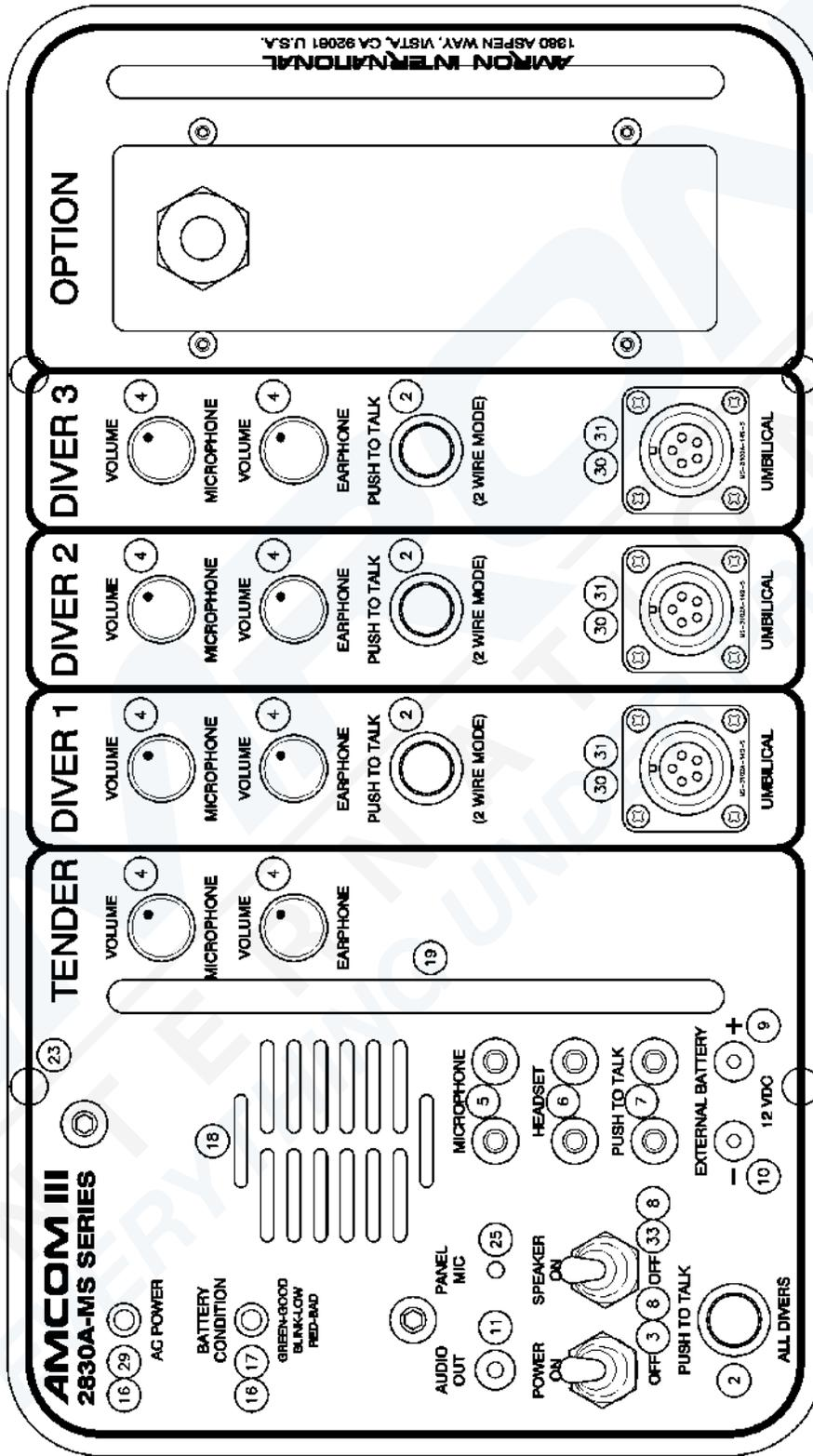
6.9 PARTS IDENTIFIER, MODEL 2830A-17, WEATHER RESISTANT AC POWER MODULE, MS CONNECTORS & DSP3 HELIUM UNSCRAMBLER
