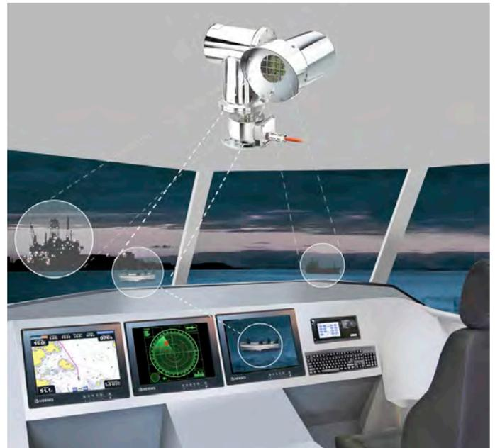
When tracking is disabled, the camera station can be controlled manually by the dedicated touch control panel HERNIS OK160, that provides smooth operation of the Radar Tracking camera and functions.
