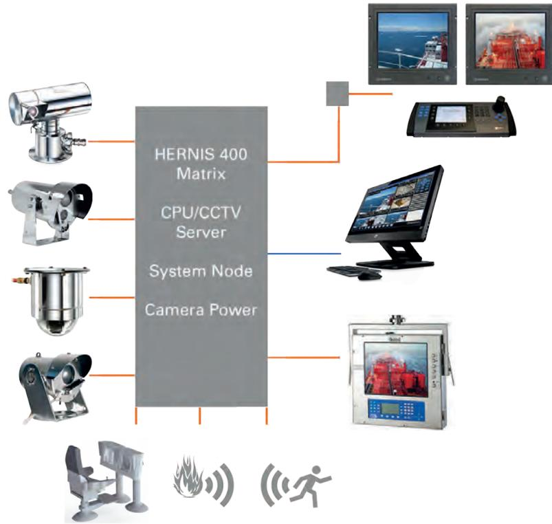
The 400 system matrix may be equipped with audio. A redundant CPU makes the system less susceptible to hardware failures thus improving the systems overall uptime. The HERNIS 400 can easily be upgraded to a hybrid system including both analogue and digital (IP
