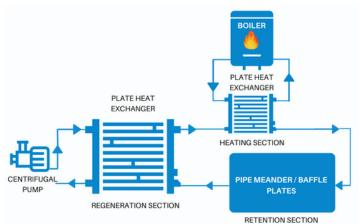
Illustration of Bawat's pasteurization technique
