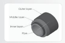
Trelleborg Offshore has many different rubber compounds that than be used "alone" or in various combinations to meet specific requirements. In addition to excellent bonding and corrosion protection of various steel, our material adheres well and can be used in combination with other polymers like:
