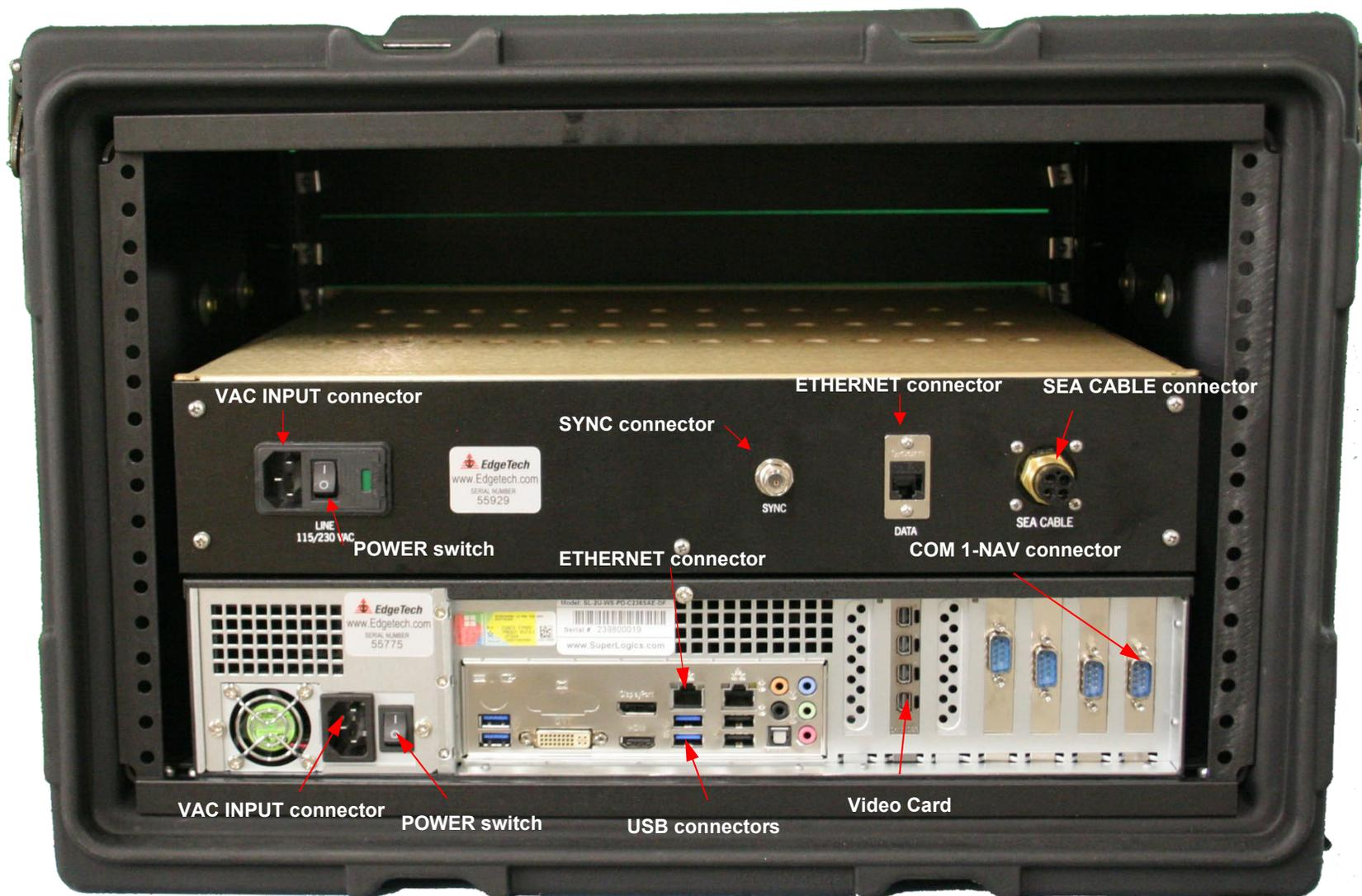
Figure 3-3: 701 DL With Computer Rear Panel
