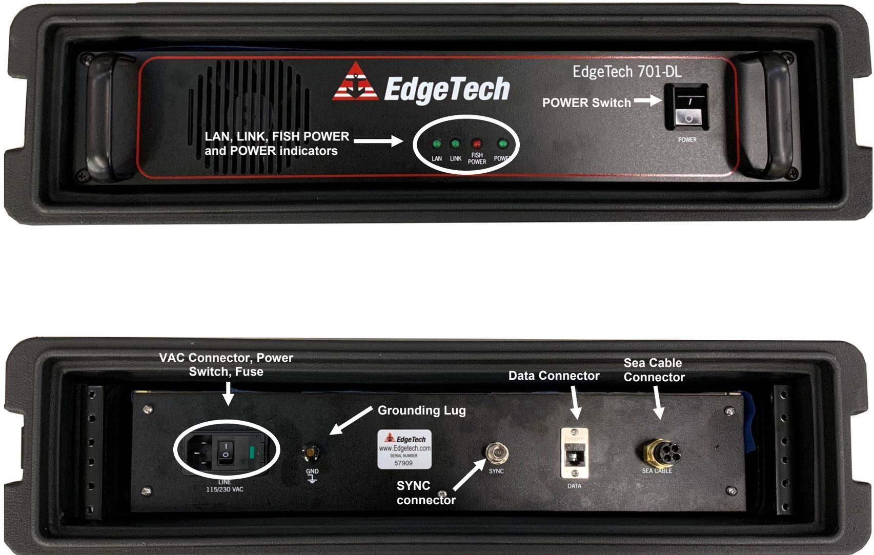
Figure 3-1: 701-DL Front and Back Panels
