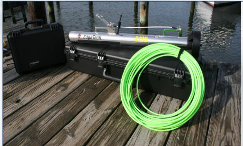
EdgeTech's 4125i Side Scan Sonar System was designed with both the Search & Recovery (SAR) and shallow water survey communities in mind. The 4125i utilizes EdgeTech's Full Spectrum® CHIRP technology, which provides higher resolution imagery at ranges up to 50% greater than non-CHIRP systems operating at the same frequency. This translates into more accurate results and faster surveys, thus cutting down on costs.
