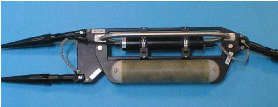
**Figure 8. Telemetry tow bar with interconnect and tow cables attached.**
