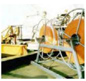
SeaSerpent DRS system positioned on deck at aft overboarding station.
