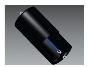
+ End fittings are M12 stainless steel eyes, connected by internal webbing strop that ease the end loads and allow suspension in any attitude from horizontal to vertical. Inflated to 0.5psi, these low-pressure fenders are robust units providing high-energy absorption, with the deflated units needing only about 10% of the normal storage space. Unique Seaflex Fenders provide a smart and tidy solution where stowage space is at a premium.
