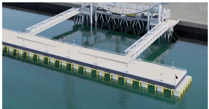
TUGDOCK's airbag buoyancy is increased and the pontoon is lifted up.
