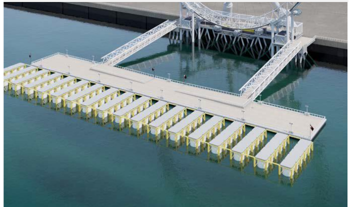
TUGDOCK frames are assembled alongside the pontoon.
