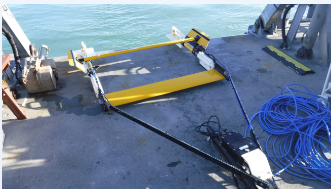
Setting the correct angle of the dihedral fins on the Geomatrix TVG Frame. Not required with 2016 TVG design..
