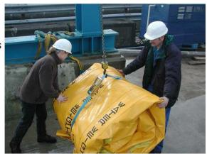
During transportation and staging, each bag including load cell, weighs approximately 1.5 % of its rated load keeping freight costs, storage space, floor loading and especially manpower to a minimum.
