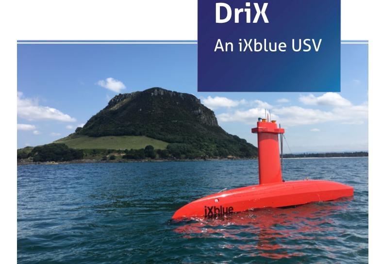
A new internationally patented 8-metre Autonomous Surface Vessel that expands your working domain and saves your vessel time.
