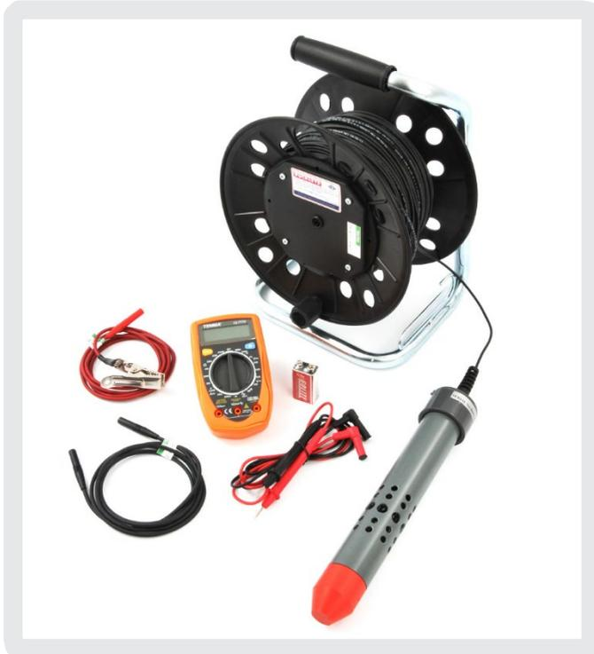
The kit has been specially created to include all items required to easily carry out a corrosion survey of marine structures.
