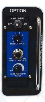
The controls for the DSP3 Helium Speech Unscrambler (HSU) are located in the options panel on the right side of the front panel as shown below.
