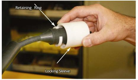
Figure 4-2: Retaining Ring and Locking Sleeve Removed
