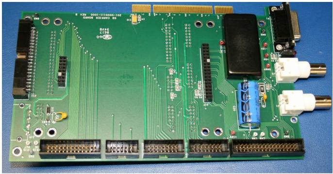
Figure 2-1: Tiger Board Set: Carrier (Front view) – 0006013
