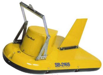
SB-216S Tow Vehicle Figure 1-3: SB-424 and SB-216S Tow Vehicles
