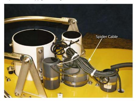
5. Push the main spider assembly pigtail through the hole in the teardrop cover in **FIGURE 4-6**.
