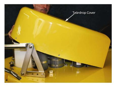
Figure 4-5: Removing the Teardrop Cover
