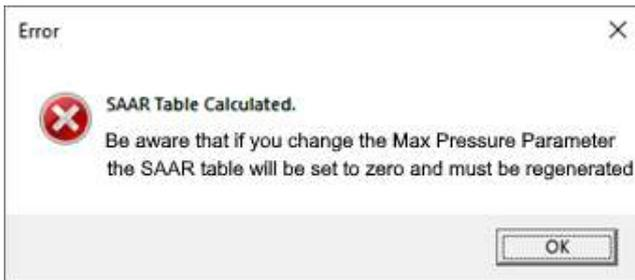
If you change the Max Pressure (dBar) setting the SAAR Table will be reset in the instrument
