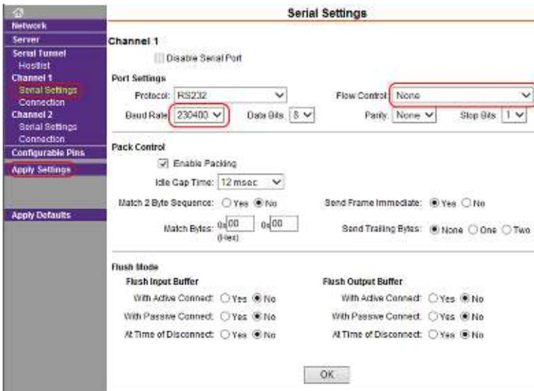
Baud Rate on Channel 1: 230400
