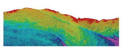
Beautiful rocky coastline off the west coast of Scotland. Data collected using an F185R+ and an R2Sonic 2024. This data was acquired in very challenging conditions - a sea state 4 with typical swell of 4.0m with up to +-16 degrees of pitch and roll. The extremely accurate performance of the F185R+ meant no editing of MBES data required. Image courtesy of Aspect Land & Hydrographic Surveys.
