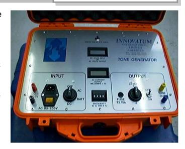
Meters are provided to monitor voltage and RMS current outputs.
