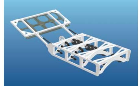
Example of job-specific tooling skid: Pipe tracking wheeled skid
