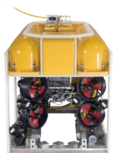
PANTHER-XT PLUS SHOWING TOOL SLEDGE COMPARTMENT
