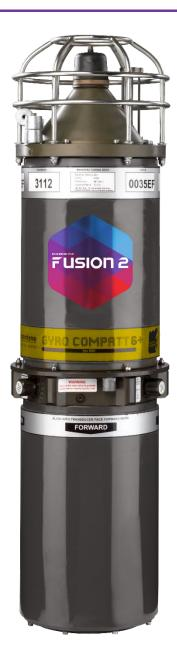
Gyro Compatt 6+ is the new industry standard, Wideband®2 and Wideband 3 acoustic positioning and Lodestar AHRS technology in one small, highly versatile and robust instrument. This provides high update rate wireless attitude, heading, heave, surge, sway, temperature, pressure, SV and acoustic positioning of any subsea object.
