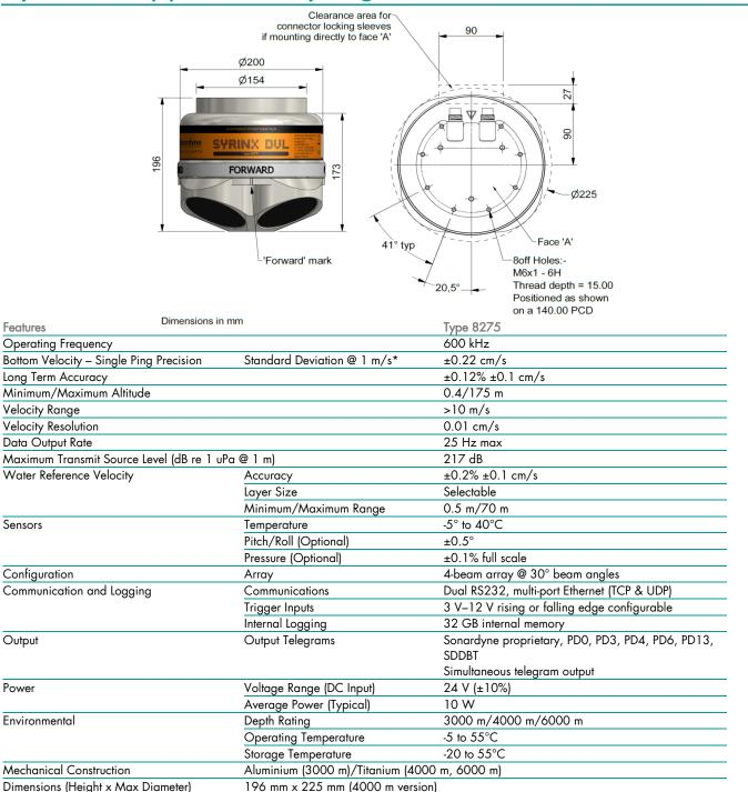
\*Standard deviation refers to proven single-ping true horizontal velocity precision, specified at 20-30 m altitude.
