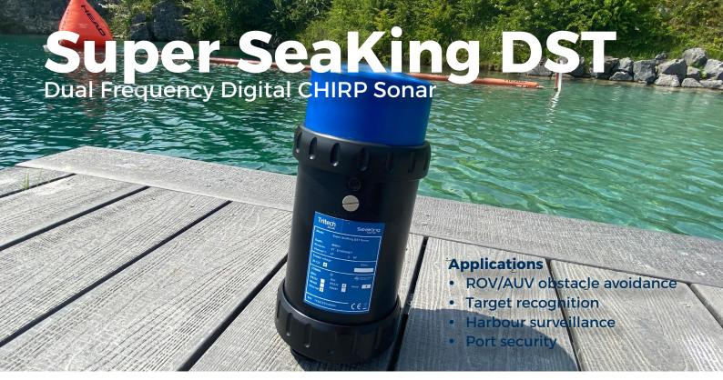
The V7 Super SeaKing DST mechanical scanning sonar now offers enhanced performance and the option of Ethernet communication for high speed scanning over short ranges. Retaining dual frequency capability, the Super SeaKing DST can achieve 300m range at 325kHz, with increased image intensity and with improved mid-water target discrimination capability at 675kHz.
