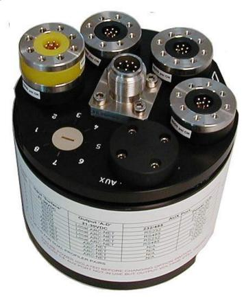
The Multicomm can be linked to a number of SeaKing sensors and communication can then be made to the Surface Control Unit (SCU) using the RS232 protocol.
