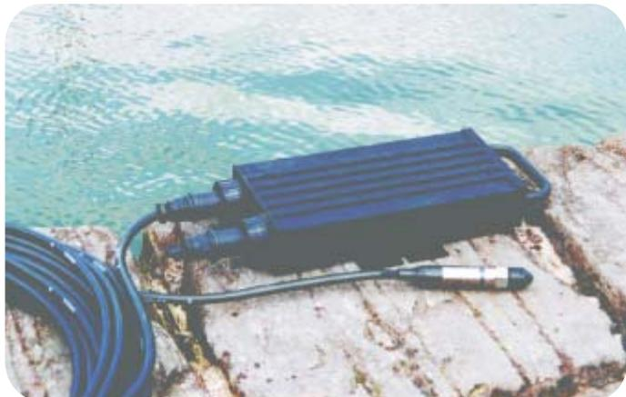
Valeport's popular Model 740 tide gauge has been designed to provide an accurate, easily deployed tide gauge for use in short or long term hydrographic survey operations. Low power consumption and user selectable sampling regime allow up to 2 years' autonomous operation, whilst the optional radio transmission package extends the capabilities for real time operations. Data output is compatible with the MIDAS Surveyor GPS Echo Sounder system.
