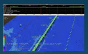
Visualisation, processing and analysis in a 3D environment leading to extensive possibilities, including automatic generation of seabed DTM, digitised pipe or cable object, calculation of free span, exposed and covered areas, as well as visualisation of events.
