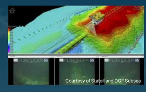
**Integration of sonar, video and tracker data** providing a detailed and complete data overview throughout the workflow, synchronised in time, position and reference. This minimises the risk of data uncertainties through continuous comparison and verification.
