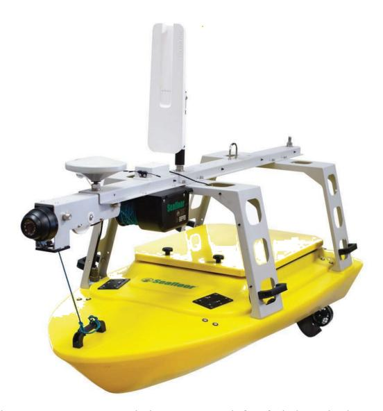
The EchoBoat-160 USV is a purpose-built remote survey platform for hydrographic data collection. With true one-switch startup, the nimble vessel accomplishes the same results demanded of large,
