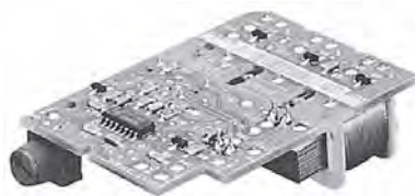
Microelectronics provide flexible and accurate motor overload protection
