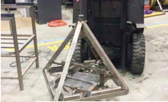
17. As the grab is raised the buckets will close, taking the sediment sample and retaining it as it is recovered to the surface.
