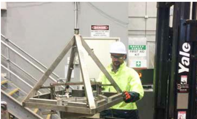
19. Guide onto the stand, taking care not to hit the buckets on the stand (this may cause the buckets to open enough to release some sample)
