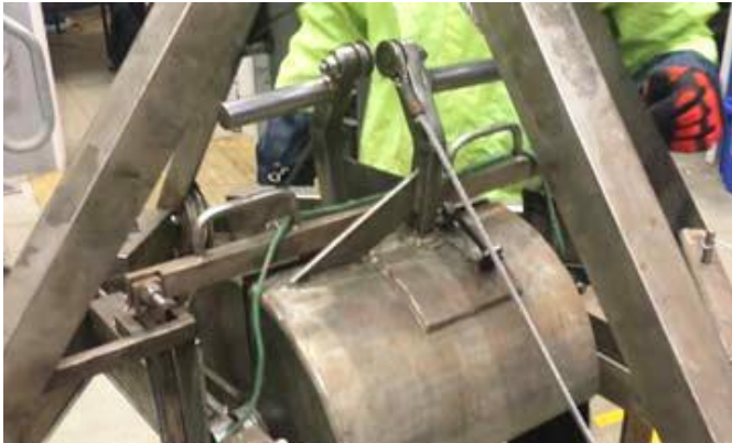
13. When trigger is lowered into place, the day grab is armed.
