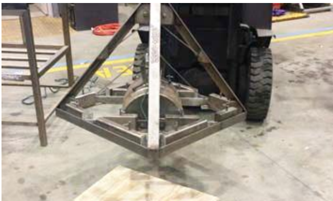
15. When the grab hits the seabed, the trigger will release the buckets.
